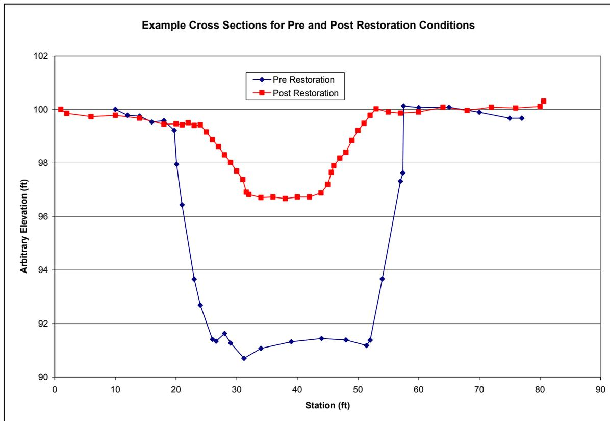
**Figure 5** – Representative cross sections of Bear Creek in the pre restoration (blue with diamonds) and post restoration (red with squares) project conditions. Notice how much larger (deeper and wider) the pre restoration channel is when compared to the restored channel.
