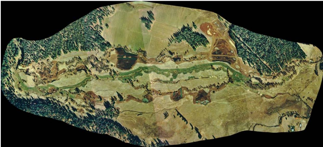
**Figure 4** – Aerial view of the Bear Creek Meadow taken in the fall of 1999, months after the construction portion of the restoration was completed. The green irrigated strip running through the middle of the meadow highlights the restored channel. The “plugged” main and secondary channels, and source ponds are distinguished by the brown color of their unvegetated earth (Photo: Hodges Aerial Photos).
